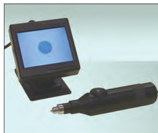
Viewer for inspection of fibre optic end face
